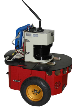
Fig. 8. A typical robot used in 2D mapping experiments. The platform is a standard ActivMedia Pioneer 2 equipped with a SICK-LMS range finder.
